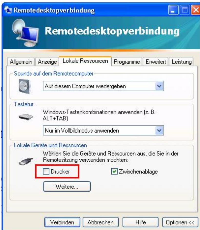
After logging on to the terminal server the session server will be started and the chosen printers will be created. On the server the client printers will be created using the naming schema "client name printer name". The advantage of this method is that the cumbersome usage of the session id for naming with the RDP protocol becomes obsolete.
